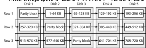
Figure 6-11 Disks in a RAID-5 volume
