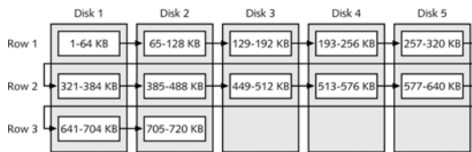
Figure 6-4 Disks in a striped volume
