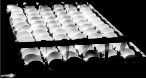
FIGURE 13-2 Candling: Eggs are automatically rolled against a light background during mass scanning, allowing checkers to remove those that have defects or that are cracked, soiled, or damaged.
