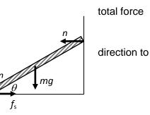
Choose the point where the ladder is in contact with the wall as the axis of rotation. Total torque equals zero:
