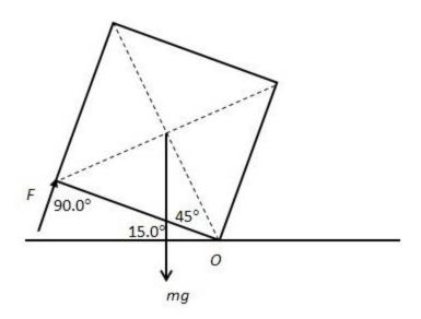
The object has a square shape and its half diagonal length is  $L\sin 45^\circ$ , where L is the side length of the object. The lever arm of gravity about point O is then  $L\sin 45^\circ\cos 60^\circ$ . So,
