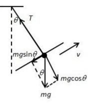
The tangential component of the bob's acceleration is equal to the rate of change of its linear speed, that is,  $a_t = dv/dt$ . The tangential component of the net force is  $-mg\sin\theta$ . The negative sign is due to the fact that this force component is opposite to the direction of motion. So,
