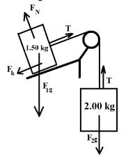
All of these equations can be combined to solve for a. Use the first to find  $F_N$  and use the definition of kinetic friction to get  $F_k$  and then solve the third equation for T and plug all of these into the second equation. So  $a = \frac{g(m_2 - \mu_k m_1 \cos 20^\circ - m_1 \sin 20^\circ)}{(m_1 + m_2)} = 3.69 \frac{m}{s^2}$
