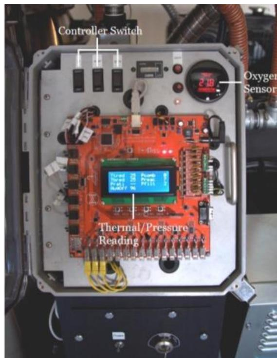
*Figure 1: Gasification Control Unit*
