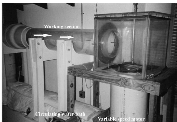
FIGURE 7.1 A “Brett”-type recirculating swim tunnel respirometer. The working section of the water tunnel houses the shark during experimentation and arrows indicate flow direction. Flow filters (not seen) within the tunnel promote rectilinear flow. A heating/cooling circulating water bath pumps heated or cooled water to regulate swim tunnel temperature. The water tunnel is currently housed at the Department of Biology, University of Mississippi, Oxford.
