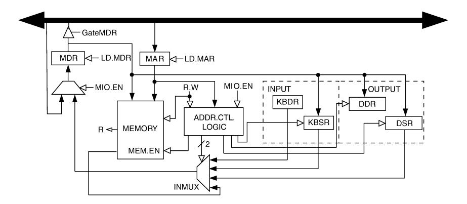
Because of interrupt enable bits, status registers (KBSR/DSR) must be written, as well as read.
